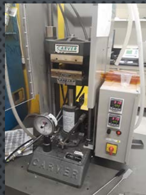
HOT PRESS (CARVER BENCHTOP) - HOT PRESS MOULDING OF POLYMERS
