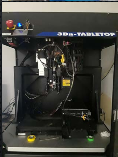
JET 3D PRINTER (NSCRIPT 3DN TABLETOP) - 3D PRINTING OF VARIOUS SOLUTIONS (WIDE RANGE OF VISCOSITY)
