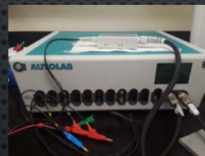
POTENTIOSTAT – EIS (METROHM AUTOLAB PGSTAT302N)
