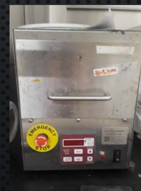
UV-OZONE CLEANER (JELIGHT UVO CLEANER 342) - SURFACE UV-OZONE CLEANING - UV-INDUCED POLYMERIZATION (OZONE-FREE LAMP)
