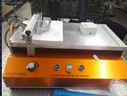
FILM APPLICATOR (ELCOMETER 4340) - UNIFORM FILM DEPOSITION (10 \mu M – 1 MM THICKNESS)
